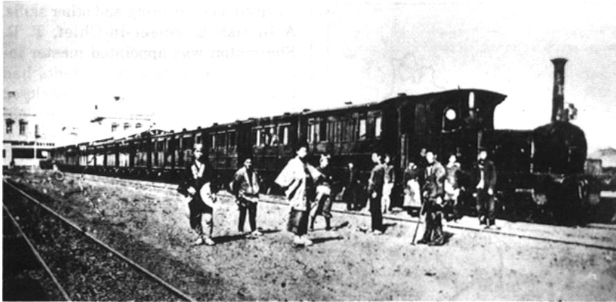
■ A tank locomotive, built by Sharp Stewart & Co., at Shimbashi Station. Courtesy: Transportation Museum, Tokyo
