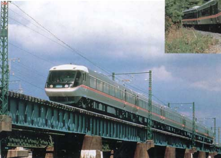
Series 383 EMU Shinano (JR Central) Shinano runs east from Nagoya and Osaka along the Chuo (West) Line to Matsumoto, Nagano and Hakuba (sites of 1998 Winter Olympics). It is a tilting train with a similar role to the Super Azusa.
