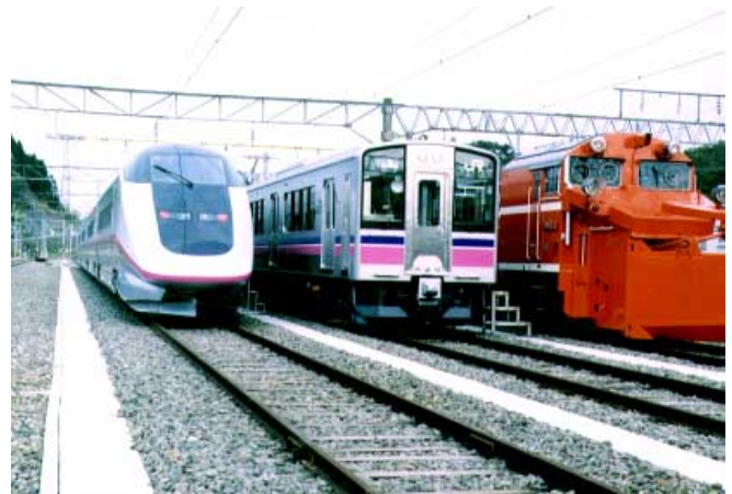
Akita Shinkansen rolling stock (JR East) From left to right: Series E3 EMU for Komachi services, Series 701 EMU for local services, and snowplowed DD18 diesel locomotive
