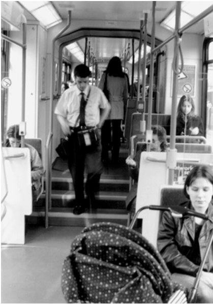
Steps between low floor and high central section of Supertram car (Author)
