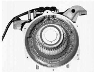
Stator of asynchronous motor. The stator is composed of a steel frame covered by coils inside. The coils are divided into three blocks: the U, V, and W phases, forming a rotating field using three-phase current from the inverter.
