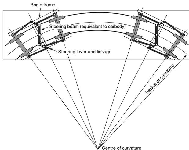
**Figure 20 Lateral Forces of Link-Type Forced Steering Bogie and Non-Steering Bogie on Rails**
