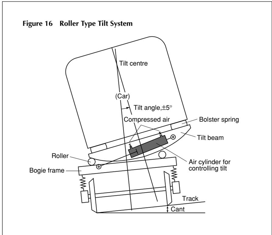
tilt railcars (Series 381) were introduced in 1973 on the western section (Nagoya to Nagano) of the Chuo Main Line. Figure 16 shows the bogie design concept. The bogie consists of a body tilting system supporting the body on two 170-mm diameter rollers and bow-shaped tilting beams with a centre of curvature aligned
