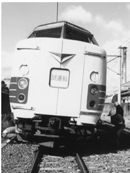
Test run of roller type controlled tilt system using Series 381 express EMU. Car body is tilted. (Author)
