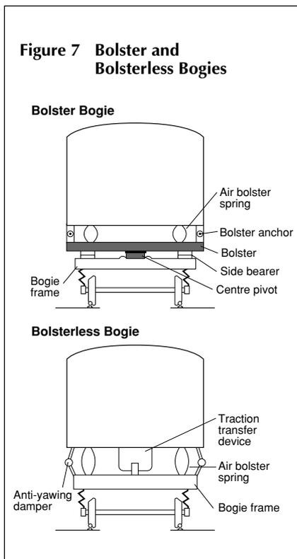
on both sides of the bogie. Rotation is resisted by longitudinal anti-yawing dampers on both sides of the bogie, resulting in better rotational resistance than conventional side bearers.
