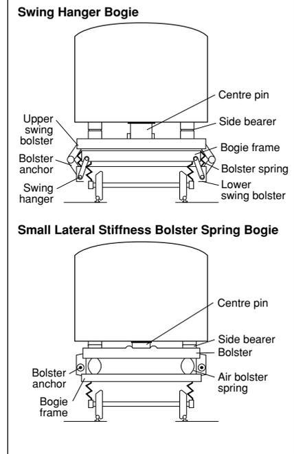
reducing the number of parts and the bogie weight (the bolsterless bogie for shinkansen was commercialized in the 1990s). In recent years, most narrow-gauge and shinkansen cars use the bolsterless bogie, which permits rotational displacement on curves through the horizontal deformation of bolster springs (also known as secondary suspension springs)
