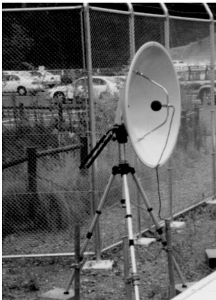
Parabolic directional microphones (RTRI)
