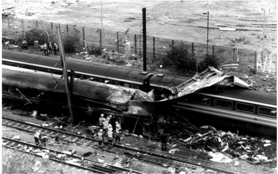
Ladbroke Grove: The dark patch of ground in front of the DMU shows where wreckage of the destroyed leading car burned after its fuel tank burst. This was the highest collision speed ever recorded for a head-on collision. (B. Morrison)
