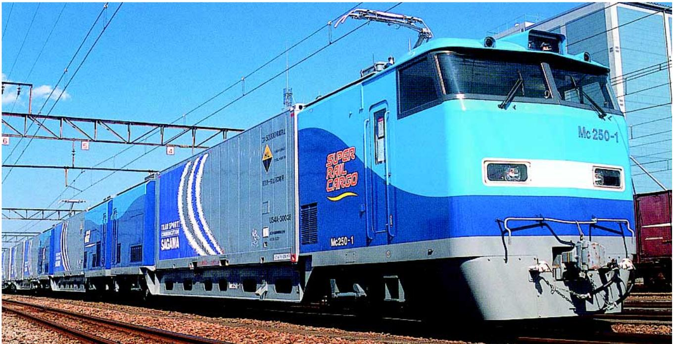
Series 250 EMU with two powered cars at each end and 12 intermediate trailing flat wagons
