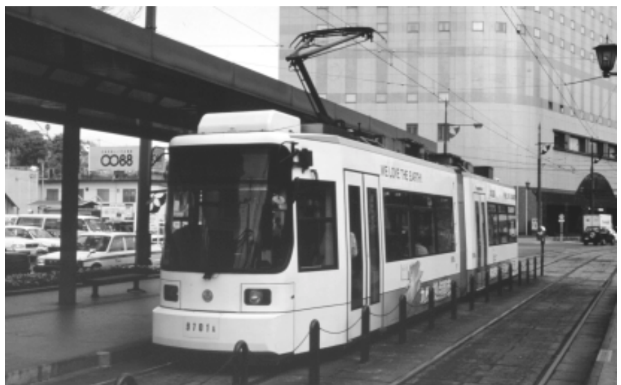
Kumamoto City's Series 9700 tram, the first low-floor car introduced in Japan in 1997. It is manufactured by Niigata Engineering, under licence from Adtranz in Germany. (Author)
