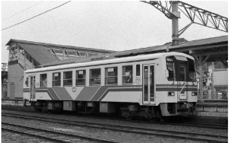
Matsuura Railway's Series MTR200 light DMU. Many railways taking over JNR's closed lines use this type of rolling stock. (Author)
