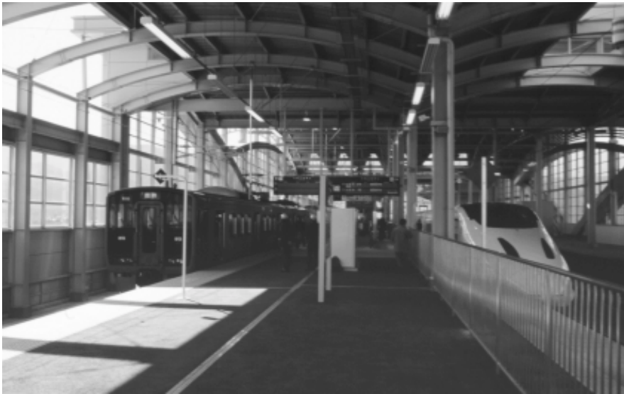
Kyushu Shinkansen's Tsubame (right) connects with a conventional train (left) at same platform in Shin Yatsushiro Station. (Author)
