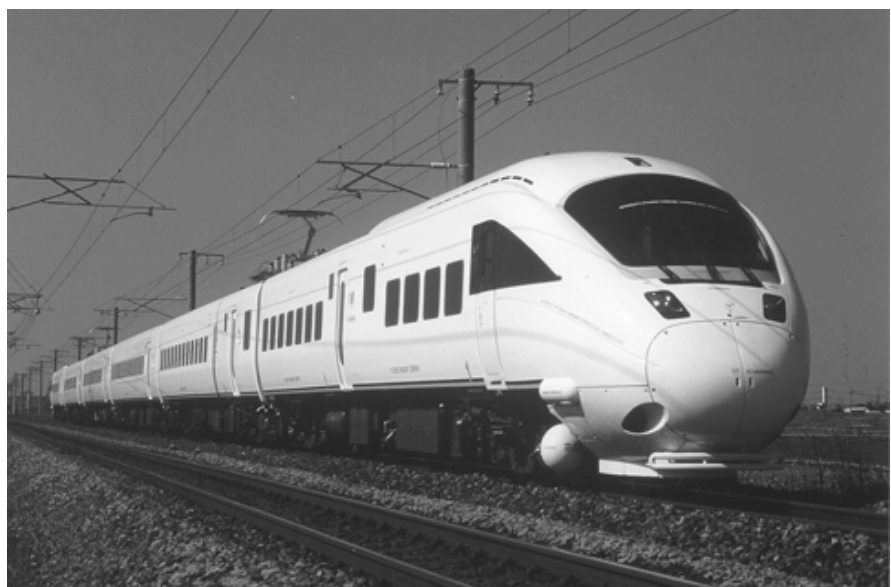
JR Kyushu's Series 885 EMU Kamome limited express. The train links Fukuoka and Nagasaki in about 2 hours with a maximum speed of 130 km/h. There is a plan to construct a shinkansen on this route, but the opening date has not been set. (JR Kyushu)
