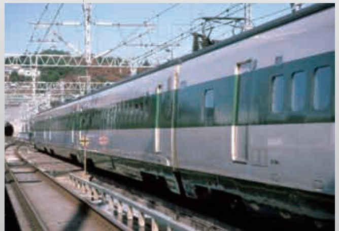
Extra bodywork to protect underbody equipment from snow
