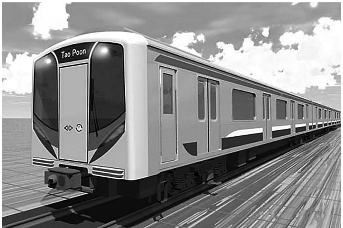
Image of three-car Sustina trainset for Purple Line
